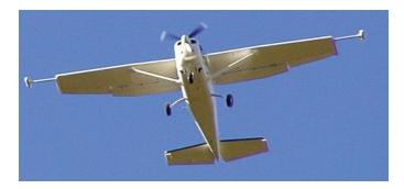
Two cesium magnetometer horizontal gradiometer system installed on a **CESSNA C206 AIRCRAFT** in wingtip pods.
