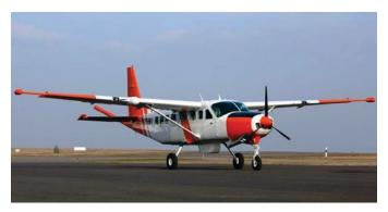
Three cesium magnetometer horizontal gradiometer system installed on a **CESSNA C208B GRAND CARAVAN AIRCRAFT** in wingtip pods and a tail-boom (stinger).
