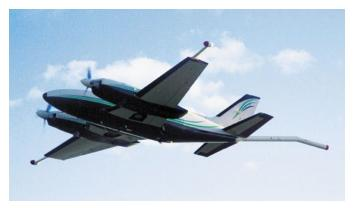
Three cesium magnetometer horizontal gradiometer system installed on a PIPER PA-31 NAVAJO AIRCRAFT in wingtip pods and a tail-boom (stinger).
